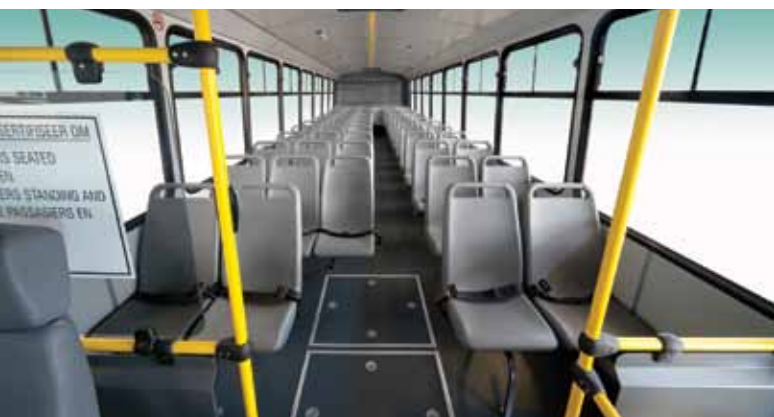
ABOVE: The standard 12,3-m long bus will accommodate 65 seated and 28 standing passengers.
