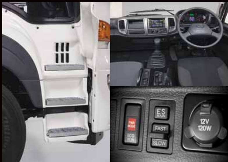
ABOVE, CLOCKWISE: Access to the cab is improved with a new step layout. The cab interior is ergonomic and of high quality. Easy Start Hill Assist is a new driver-assistance feature. LEFT: Ready for the drive!
