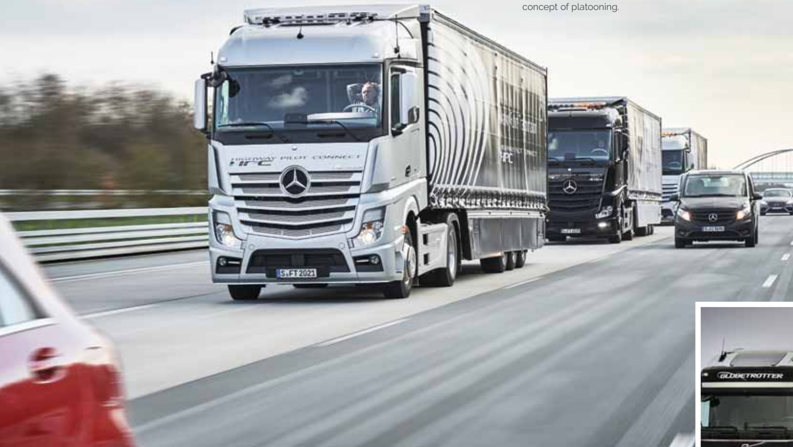
Mercedes-Benz Actros demonstrates the concept of platooning.
