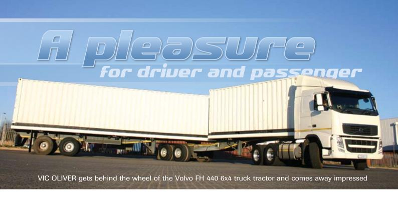
ur **FOCUS** Volvo FH 440 6x4 truck tractor test unit was coupled to a set of flat-deck inter-link trailers complete with fully loaded 6 m and 12 m ISO containers, bringing the total gross mass of the rig to 53 740 kg.
